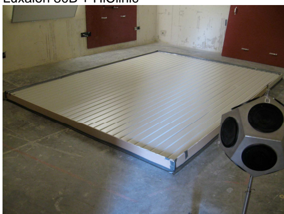
Measurement set up, construction height 100 mm
